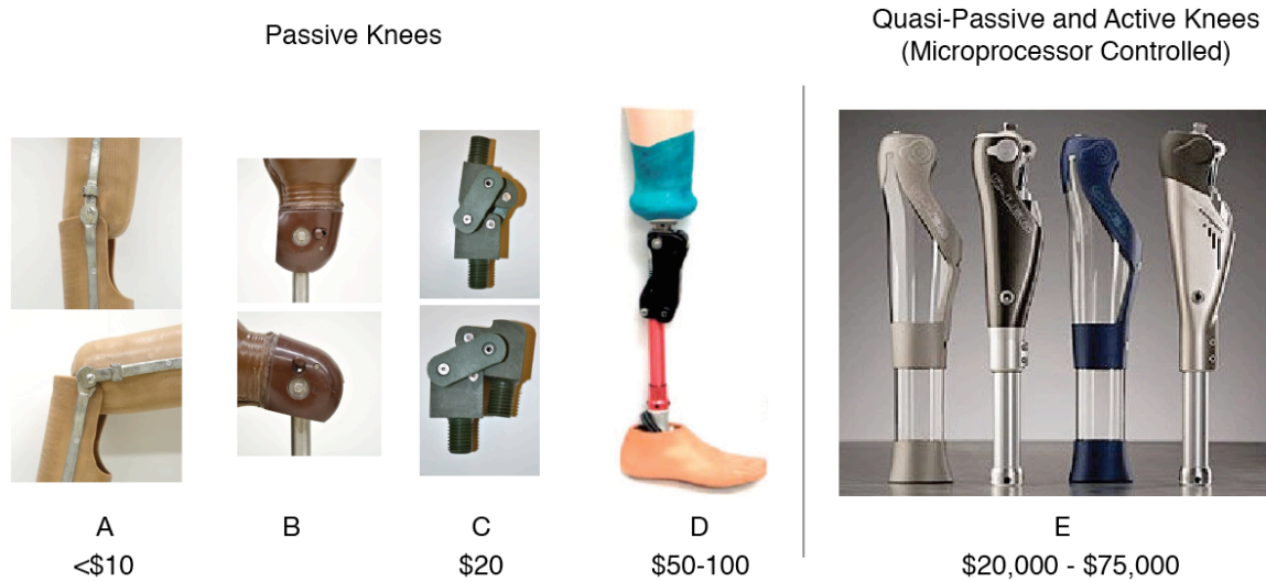
Figure 1. Different Prosthetic knees available in the developing and developed world markets and their selling prices: A) BMVSS (Jaipur-foot) manual-locking knee, shown fully extended and at full flexion [22] B) The International Committee of the Red Cross (ICRC) manual locking, single-axis knee C) Jaipur-Stanford four-bar knee joint used by BMVSS [3] D) LCKnee designed by J. Andrysek [14], with an automatic locking mechanism E) The popular Ottobock range of quasi-passive and active, microprocessor-controlled prosthetic knees: C-leg and Genium Microprocessor controlled knees have been widely adopted in the developed world markets and they can enable a wide range of activities and motions [13].
