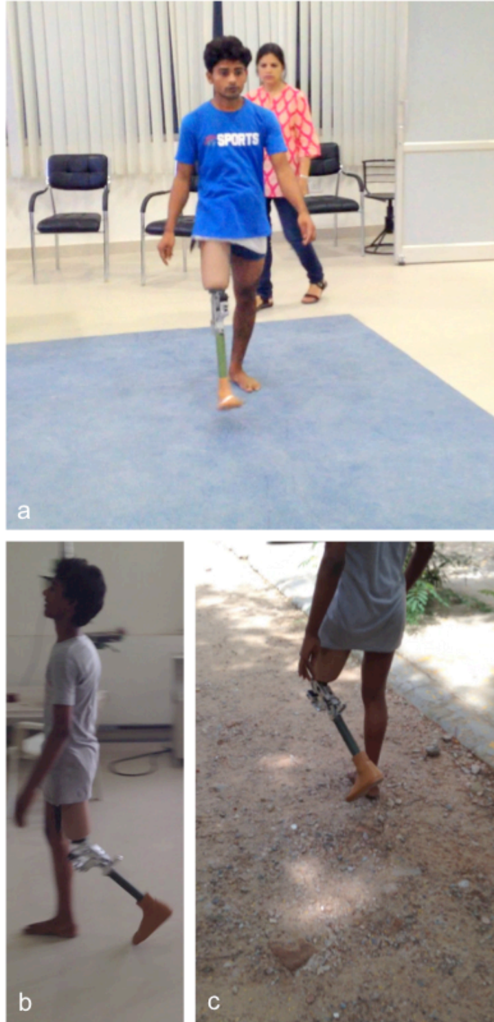
Figure 5. PRELIMINARY FIELD EVALUATION. 4a. Subject 1 using the prototype for the 2-minute walk test. 4b. Subject 2 during the 2-minute walk test, late stance flexion of up to 40 degrees can be seen. 4c. Subject 2 walking comfortably outdoors on a relatively flat, muddy terrain.
