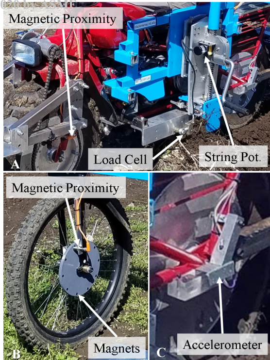
Fig. 11. CLOSE-UP VIEWS OF SENSOR INSTALLATION EXAMPLES. Views of prototype shown are (A) left-side, (B) outrigger wheel right side, and (C) rear axle left side
