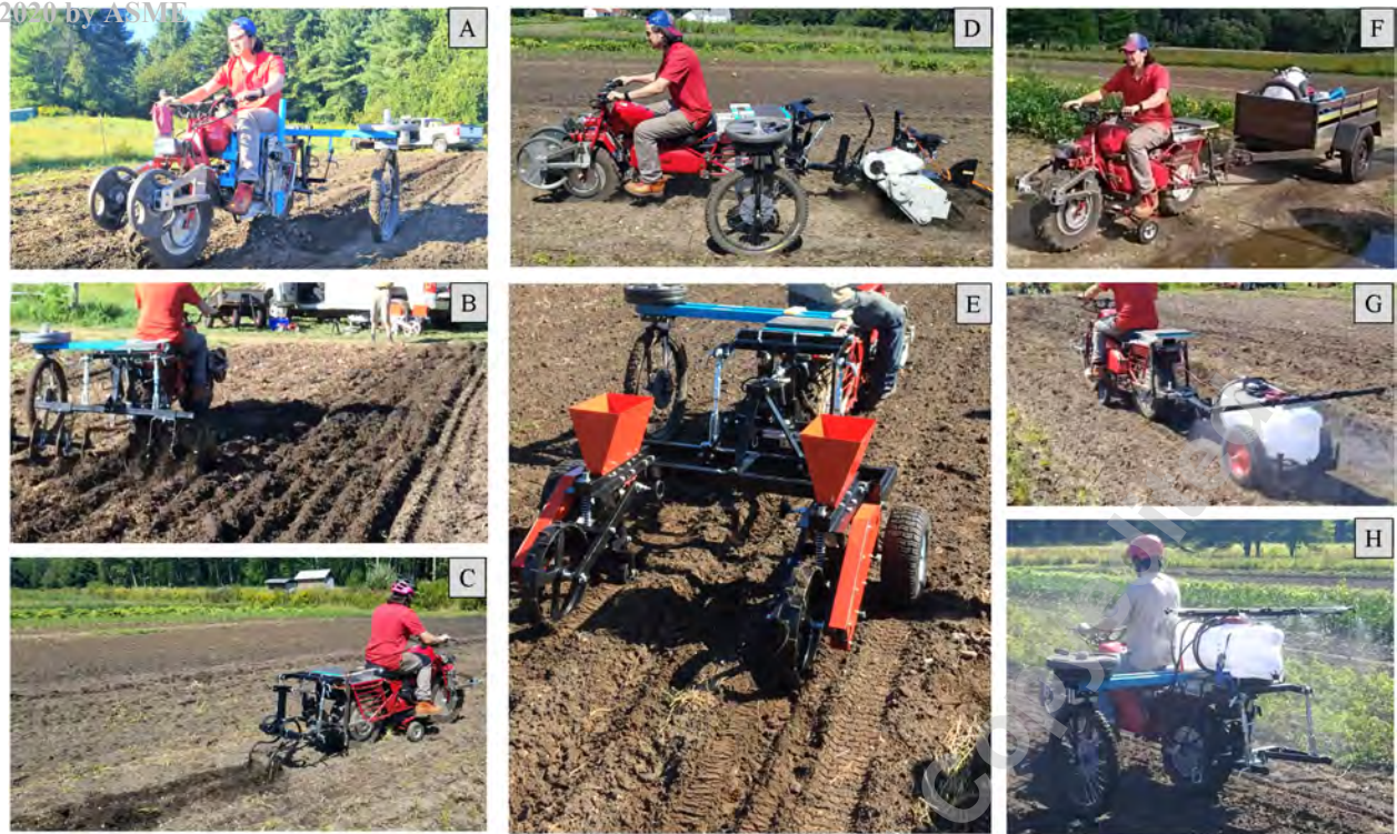
Fig. 7. IMAGES OF THE RESEARCHERS PERFORMING KEY OPERATIONS OF INTEREST TO INDIAN FARMERS WITH BULLKEY. A) Plow B) Disc harrows C) Cultivator D) Rotavator E) Planter F) Trailer G) Sprayer on its trailer H) Sprayer on motorcycle.
