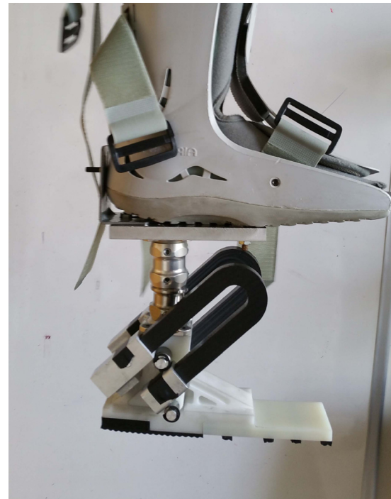
Fig. 11 Pseudo-prosthesis boots mounted with the prosthetic foot prototype for preliminary testing
