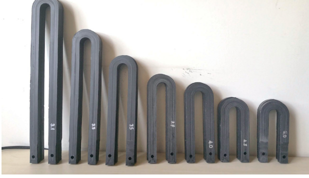
Fig. 7 Set of springs with different rotational stiffness values. The longer the spring, the more compliant it is.
